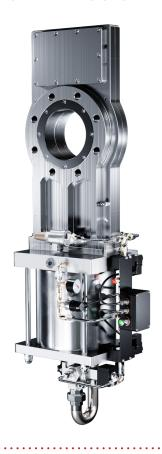
The GatEx PRO quick-acting slide valve is part of a system used to prevent the propagation of an explosion between the individual units of the production technology. When an explosion occurs, the pipe will be completely closed in milliseconds.
