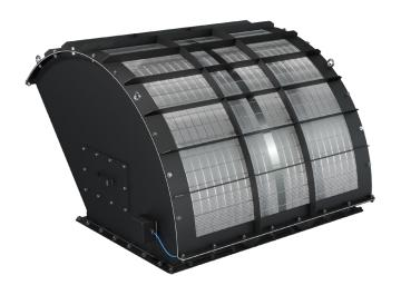
This is a safety device designed to relieve and release explosions developing inside a protected device that is in an explosive environment. In the event of an explosion, FLEX captures the explosive energy (flame, pressure) emerging from the open explosion relief device. Thanks to the special design of the flame filter, it cools the temperature of the flame and exhaust gases during the explosion to a level that is no longer dangerous to technology and to people in the proximity.
